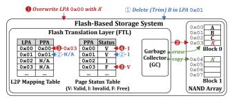
Figure 3. An illustrative example of how an FTL works.
