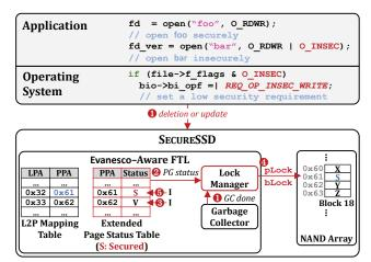
Figure 13. Operational overview of SecureSSD.
