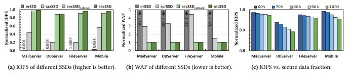
Figure 14. Performance of SecureSSD under four different workloads.
