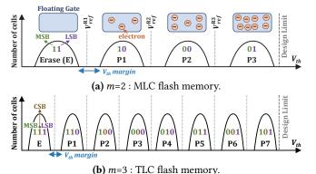
**Figure 2.**  $V_{th}$  distributions of  $2^m$ -state NAND flash memory.
