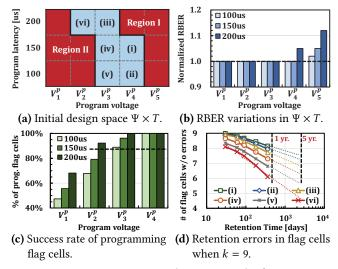
Figure 9. Design space exploration results for pLock.
