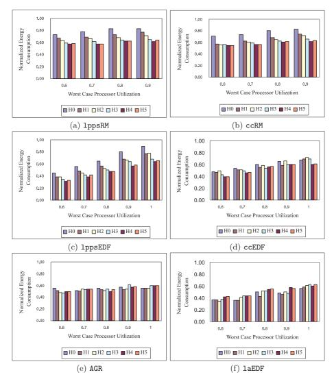
Fig. 6. Energy efficiency comparison results of the HybridDVS algorithms
