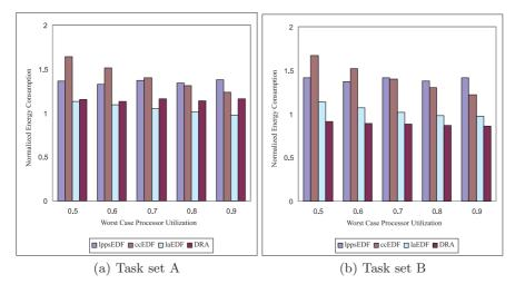
Fig. 4. Normalized energy consumption of InterDVS algorithms over intraShin
