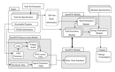
Fig. 2. An overview of the SimDVS simulation environment
